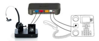
Please be aware that the device will not be fully functional until the colored markings for all cables have been connected to the EHS adapter, see photo.
